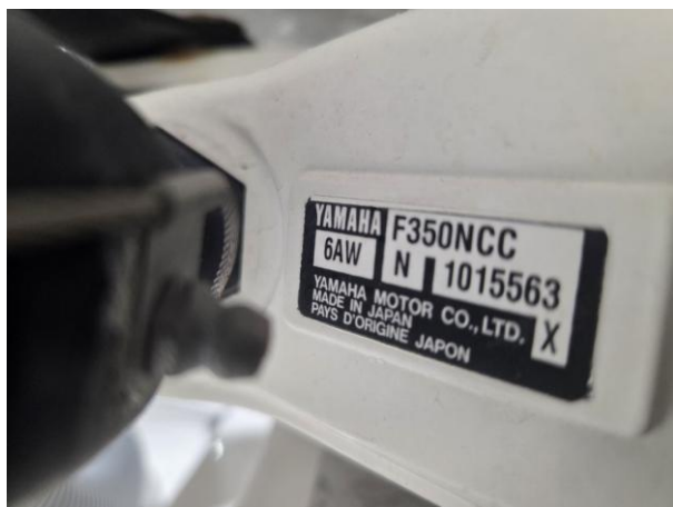
07 Port engine data plate: Yamaha F350NCC, 6AW N 1015563.
