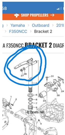
59 DEF-2: Reference — Yamaha F350NCC 'Bracket 2' parts diagram identifying the affected steering-arm bracket and fasteners.
