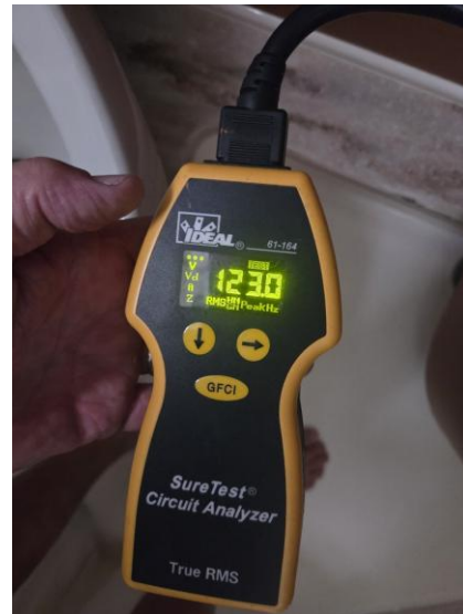
37 Generator peak output tested good (circuit analyzer).
