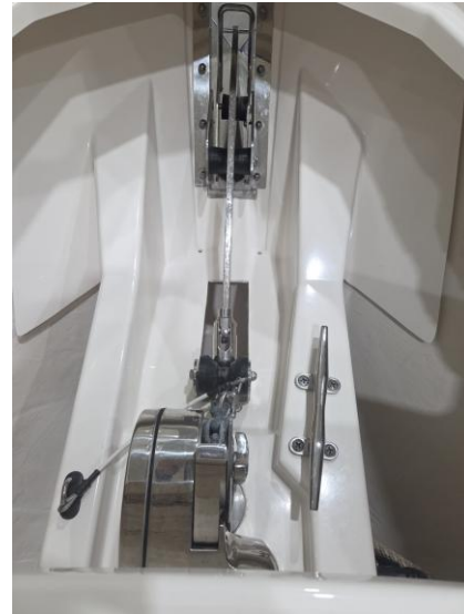
33 Lewmar stainless windlass operated up/down from helm and bow remote.
