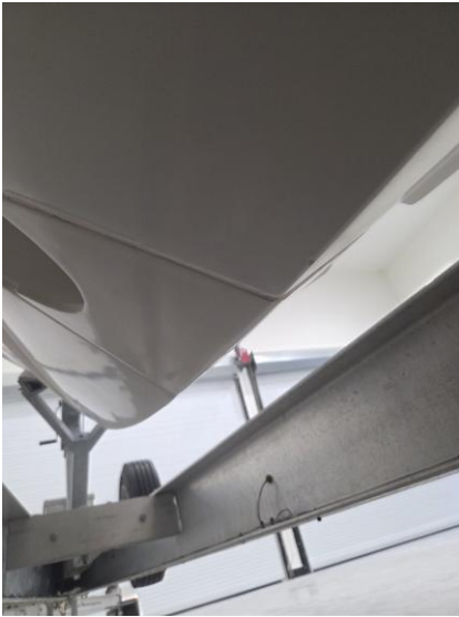
03 Hull examined out of the water by phenolic-hammer sounding and Tramex Skipper moisture meter; no blistering, delamination, significant abrasion or prior damage sighted.
