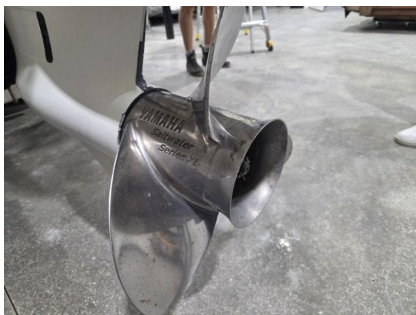
11 Yamaha Saltwater Series XL stainless propeller (17 x 16.25).
