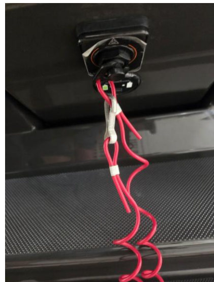
16 Engine emergency cut-off (kill) switch operated.
