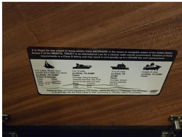
46 Overboard-discharge (MSD) placard displayed.
