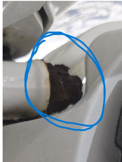
58 DEF-2: Severe corrosion on the steering-arm connection clamp, typical of all three engines.
