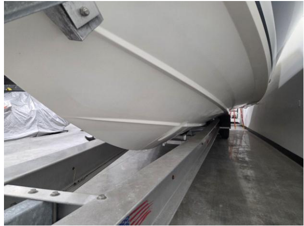
04 Hull bottom clean; bare gel coat, no antifouling; no damage sighted.
