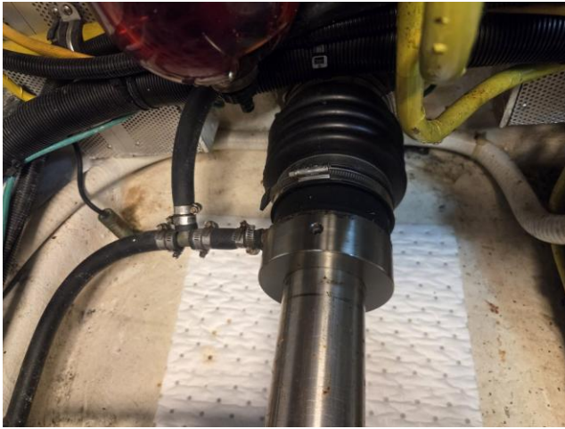
31 Dripless shaft seals in good serviceable condition
