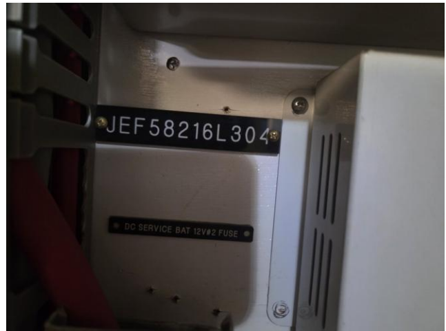
02 Hidden HIN plate on the engine room forward bulkhead
