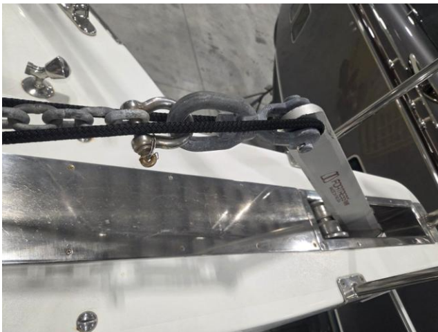
77 Anchor terminal connection — properly safety-wired
