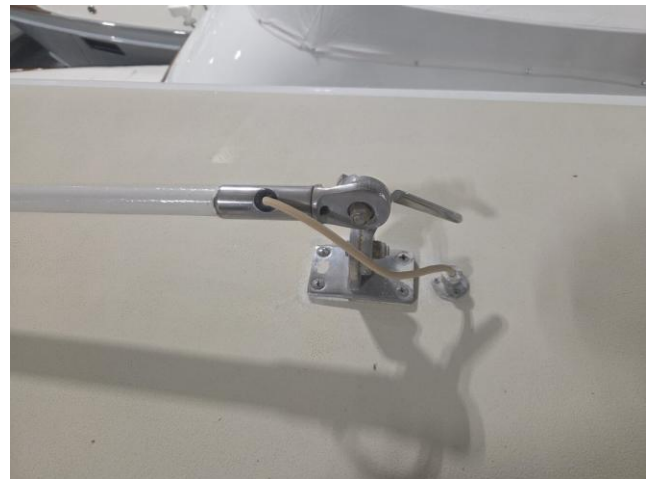
50 Antennas well secured on adjustable stainless mounts
