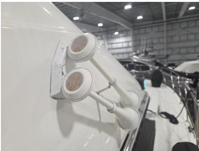
59 USCG-approved dual compressed-air horn sounded
