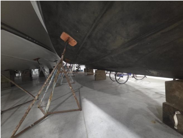
11 Bottom sounded with a phenolic hammer — no delamination
