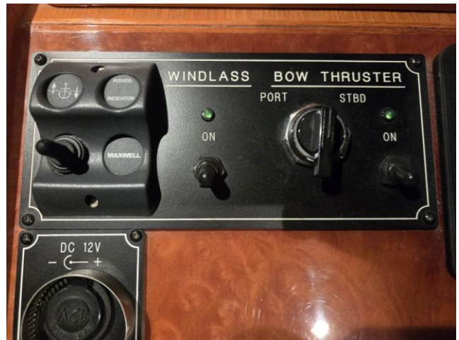
78 Windlass and bow thruster controls at both helms and the bow
