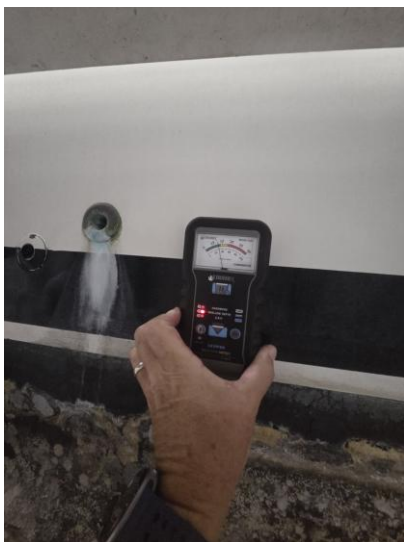
09 Moisture meter readings taken along the topsides
