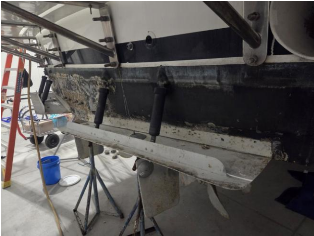
13 Trim tabs clean with proper cathodic protection
