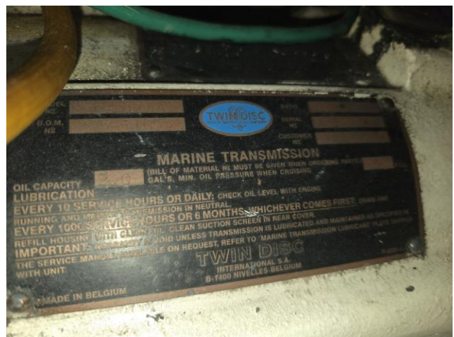
24 Twin Disc marine transmission data plate
