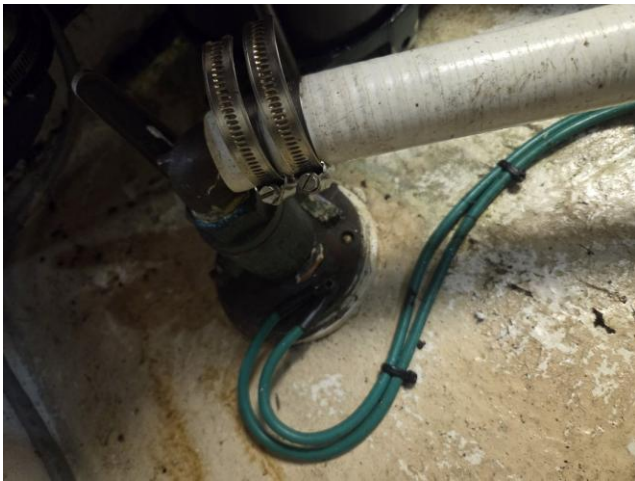
69 Seacock and bonding conductor
