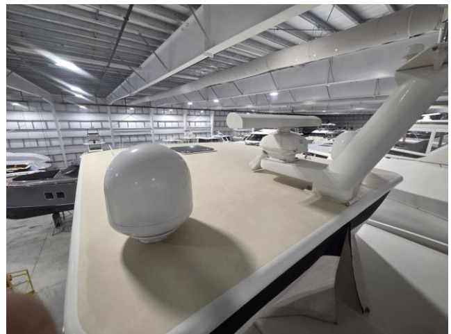
60 Hardtop — radar and satellite dome
