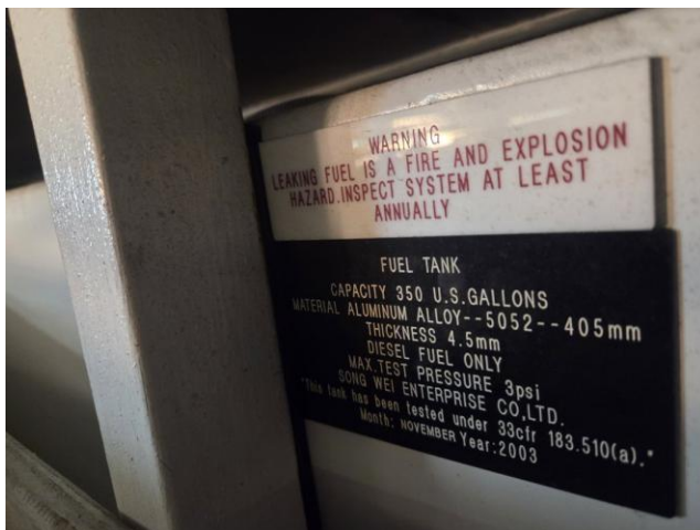
61 Fuel tank label — 350 U.S. gal, 5052 aluminum, tested to 33 CFR 183.510(a), Nov. 2003
