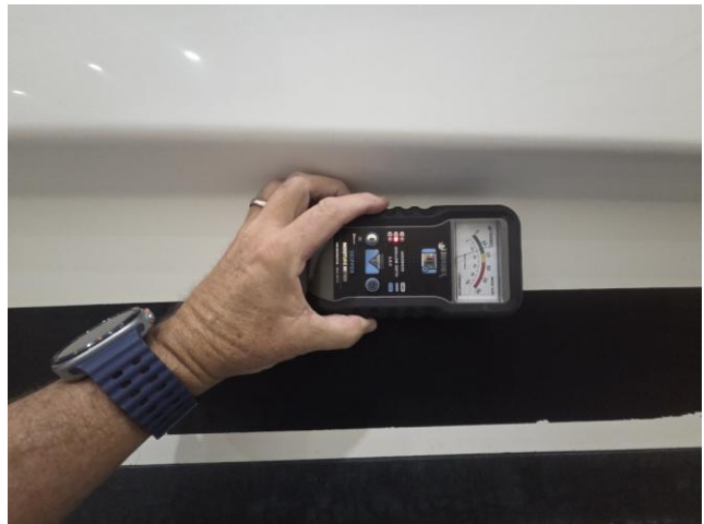
08 Hull and transom metered — no elevated moisture above or below the waterline
