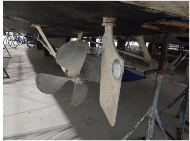
32 Props, shafts and rudders well maintained — no significant corrosion or growth
