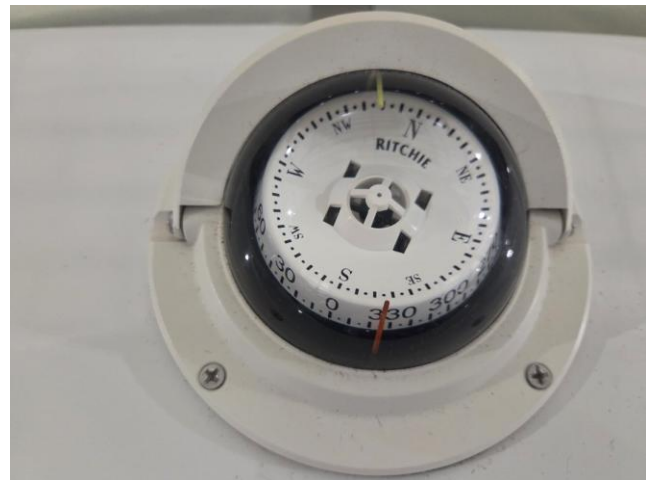
54 Ritchie magnetic compass — upper and lower helms appear accurate
