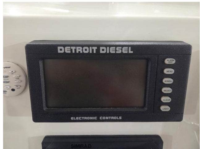
48 Cockpit station DDEC display and Simrad autopilot
