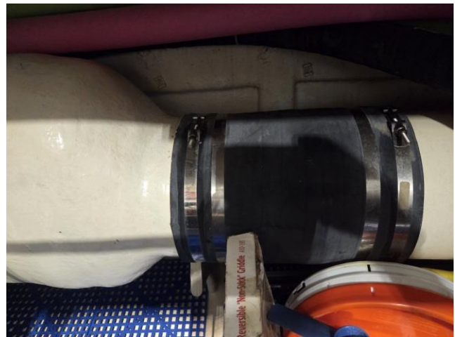
28 Exhaust hose connection double-clamped
