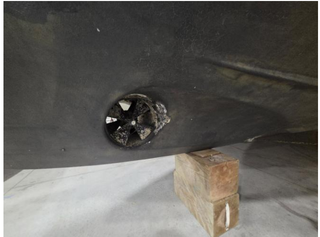
14 Bow thruster tunnel and props
