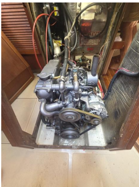
24 Yanmar 3HM35F — ran well during the sea trial
