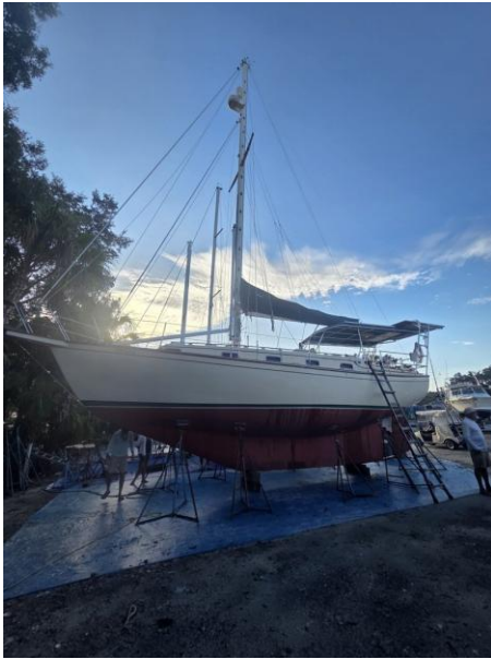
06 Vessel inspected out of the water — port side profile. Hull bottom tested with phenolic hammer and moisture meter, no exceptions
