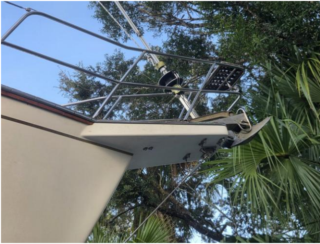
10 Hull-integral bowsprit — very solid
