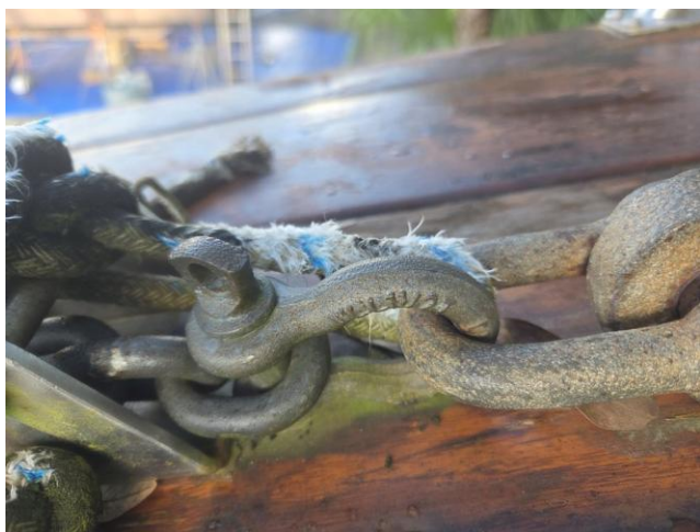
67 DEF Anchor shackle has no safety wire (mousing)
