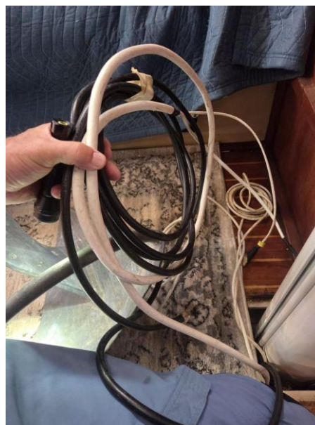
23 DEF Mast wiring not routed into the mast
