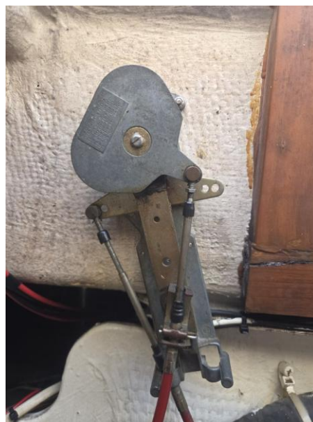
35 DEF Throttle / shift mechanism requires adjustment, lubrication or replacement
