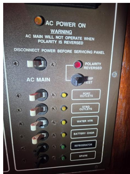
38 AC main panel well marked, with reverse-polarity indicator
