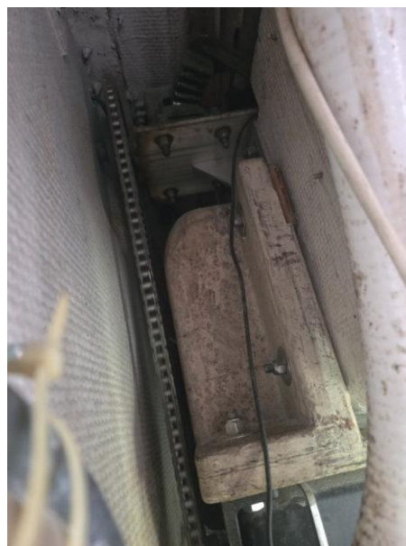
33 Autopilot drive appears well adjusted and lubricated
