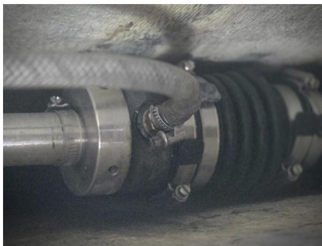
31 Dripless shaft seal — leaked on launch, diminished after 20 minutes in gear
