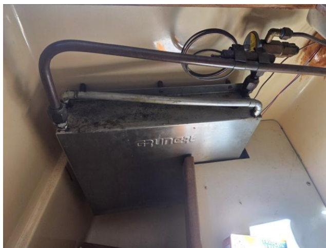
62 Galley refrigerator / freezer operates on 120 VAC shore power only
