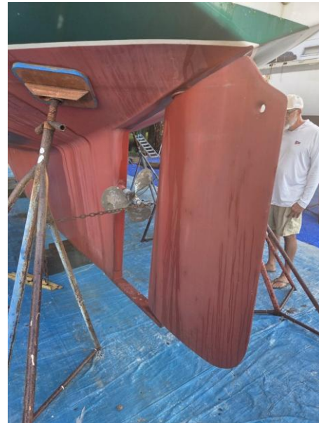
09 Rudder in very good condition; operates through full range
