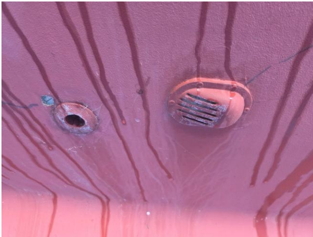
08 Hull bottom clean; thru-hulls clean and corrosion-free
