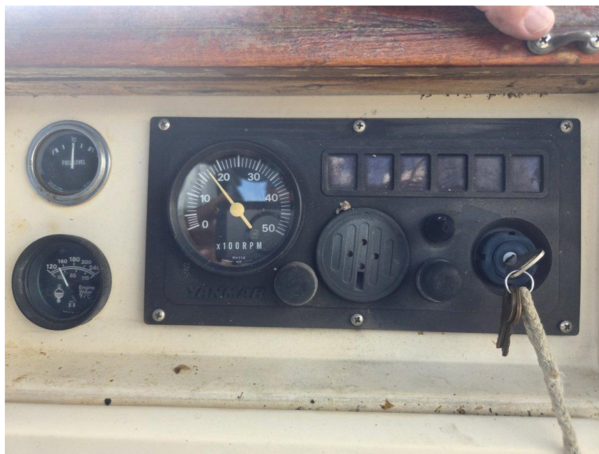
36 Engine panel: start, tachometer, fuel gauge and engine temperature. No oil pressure gauge installed
