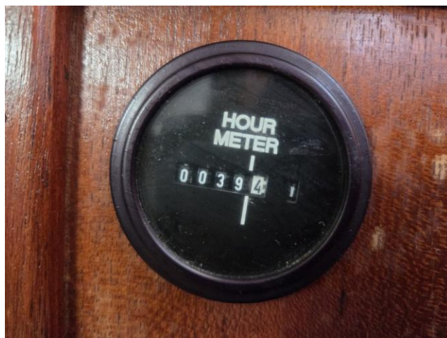
26 Second hour meter — approximately 394 hours (may indicate hours since rebuild)
