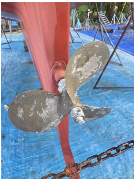
32 Three-blade bronze propeller (est. 16 x 14; no legible marking); no significant impact damage or corrosion
