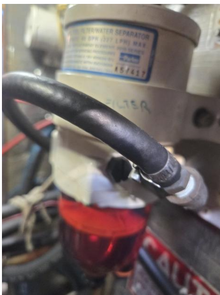
30 Racor fuel filter / water separator clean
