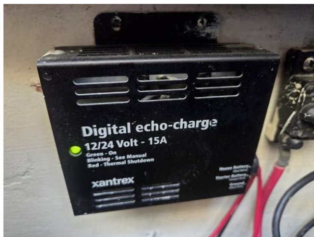
45 Xantrex Digital Echo-Charge — status light green
