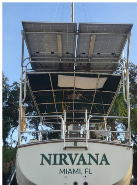
46 Stern profile — solar panel support frame very secure and well designed
